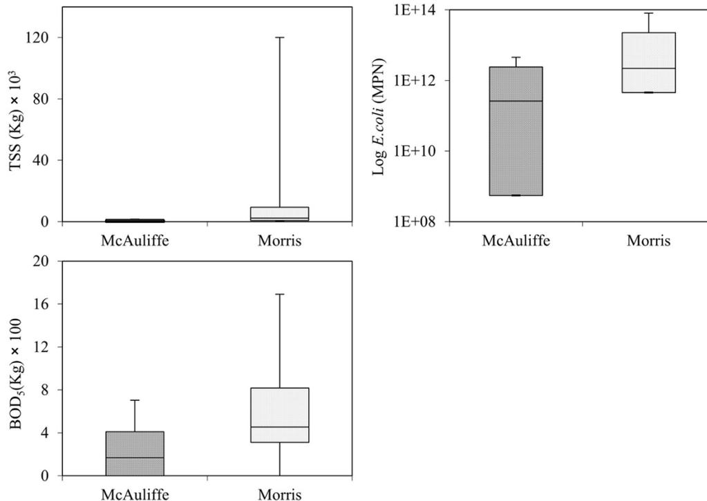
**Figure 6.** Box and whisker plot for different pollutant load at the outlet at McAuliffe and Morris RDFs.
