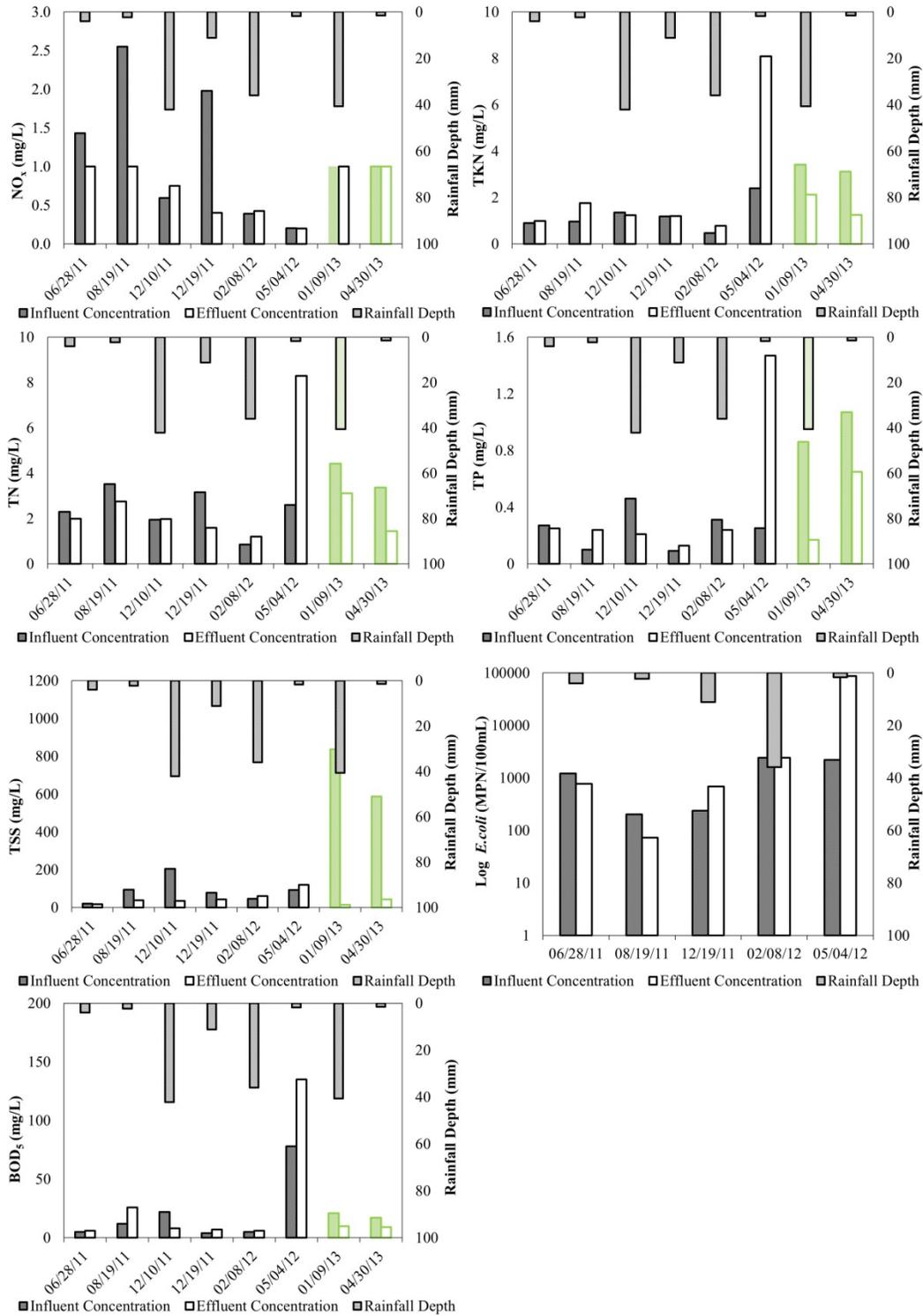
**Figure 5.** Influent and effluent concentrations (mg/L) for different pollutants collected at McAuliffe RDF at different rainfall depths, green bars indicate the samples collected after the microscreen installation.
