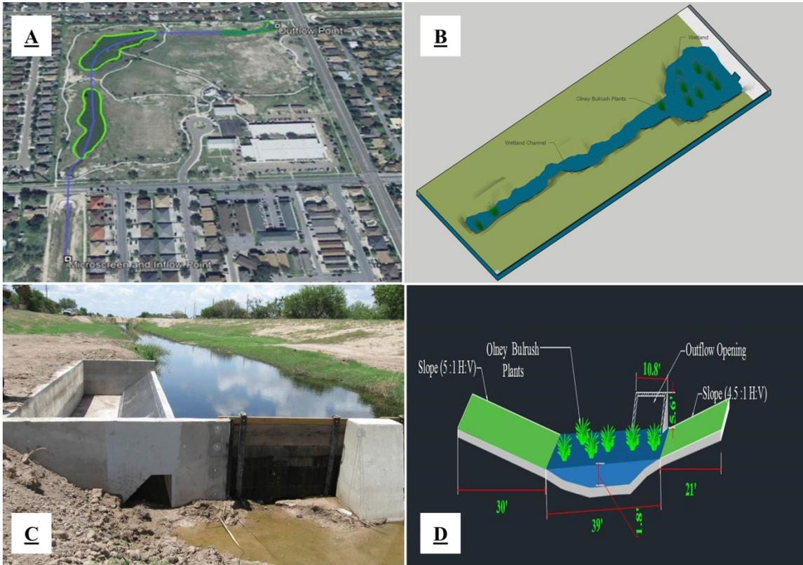
**Figure 1.** McAuliffe Regional Detention Facility (RDF) site: (A) site location showing the two wet detention and wetland locations, (B) wetland structure, (C) microscreen installed at the inlet, and (D) cross-section showing the depth and dimensions of the McAuliffe wetland.
