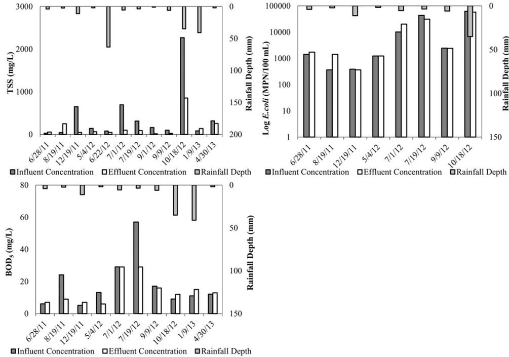
**Figure 4.** Influent and effluent concentrations (mg/L) for different pollutants collected at Morris RDF at different rainfall depths.
